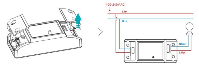
· Make sure all wires are connected correctly
