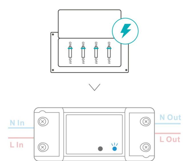
\*The device will exit the Pairing Mode if it is not paired within 10mins. If you want to enter this mode again, please long press the button for 5s until the LED indicator flashes in a cycle of two short and one long and then release.
