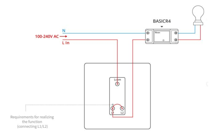
**Note:** Only compatible with mainstream brands of double pole rocker switches Rocker switches. The rear-end light needs to be compatible with mainstream brands of LED, energy-saving lamps, and incandescent lamps ranging from 3W to 100W.
