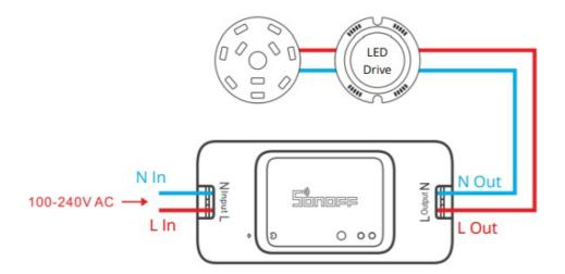
Make sure the neutral wire and live wire connection is correct.
