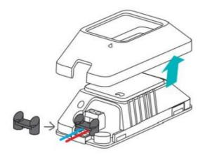
To remove the protective cover, then connect wires before fixing the wire fastener. installation, please align " " with " " when securing the protective cover.
