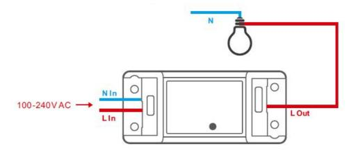
Make sure the neutral wire and live wire connection is correct.
