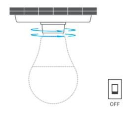
• To avoid electric shock, please turn off the power before installing the device.
