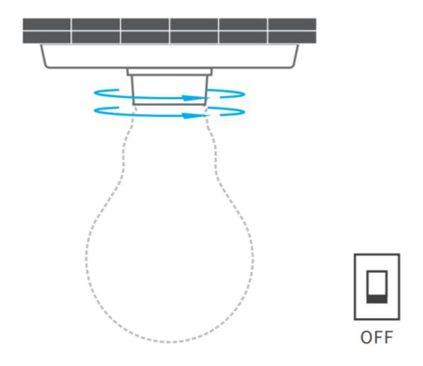
riangle To avoid electric shock, please turn off the power before installing the device.
