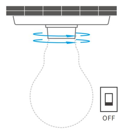
To avoid electric shock, please turn off the power before installing the device.
