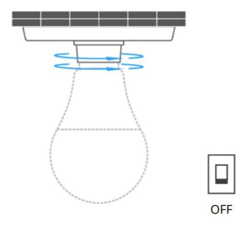
To avoid, electric shock, please turn off the power before installing the device.
