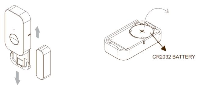
4. Note to distinguish between the + or – of the battery, install the new battery in the battery compartment correctly, and push the compartment into the sensor, then check and make sure that the battery compartment got locked and secured.
