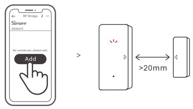
Access the eWeLink APP and select the Bridge, tap "Add" to select the alarm, and a "Beep" means the Bridge enters the pairing mode. Then seperate the magnet for more than 20 mm from the transmitter until the LED indicator stays on for 1 to 2s, and the pairing is complete when you hear "Beep Beep".
