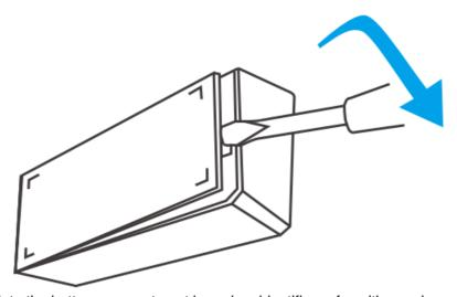
2-2. Insert batteries into the battery compartment based on identifiers of positive and negative poles.
