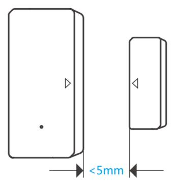
Make sure the installation gap is less than 5mm when the door or the window is closed.
