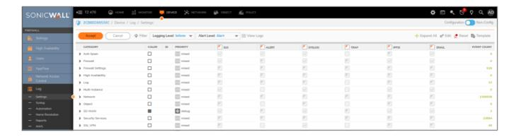
The Device > Log > Settings page displays logging settings in a series of columns and allows you to configure the logging and alert levels, edit attributes of all categories, groups, and reset all event counts. You can filter the entries to limit the data display to only those events of interest. You can select storage options on appliances with built-in or flexible storage components, and you can import and save logging templates.
