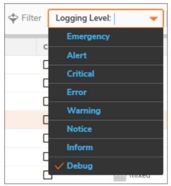
On the Log > Settings page, you can set the baseline logging level to be displayed on the Monitor > Logs > System Logs page. The following logging levels are available for selection, from highest to lowest:
