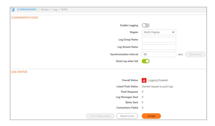
Logged events generated on the firewall can be sent to the AWS CloudWatch Logs service. From there, the data can be used by AWS hosted analysis tools such as ElasticSearch and Kibana.
