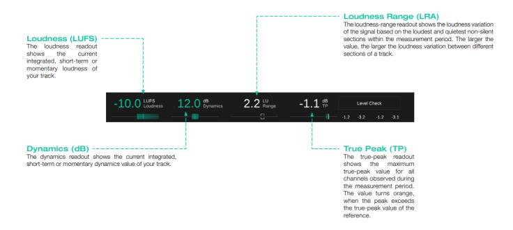
true: level is using the median of all measured PSR (peak to short-term loudness ratio) values for measuring the dynamics of a track. Compared to the well-known PLR (peak to long-term loudness ratio) value used by other tools, our experiments showed that our PSR based descriptor better traces the actual dynamics of a track, including short-term dynamics.
