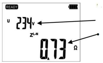
6. The value of short-circuit current lk and of individual impedance components ZS (R, XL) may be read when pressing the up or down arrow buttons for indications dis-played in reverse order
