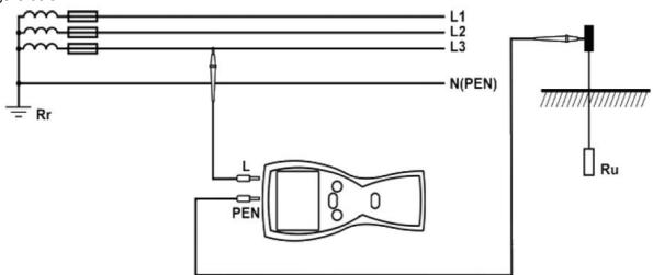
During the measurement, check the connections of the measured earth electrode with the electrical installation. For correct measurement, the tested earthing system should be disconnected from the electrical installation (N and PE conductors). If you want to measure the earth electrode, for instance in the TN-C-S system and
