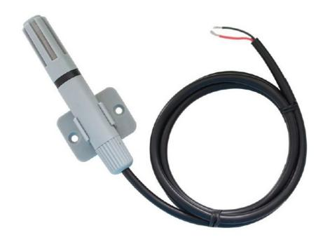
SM7330M using the standard,easy access to PLC DCS and other instruments or systems for monitoring temperature, and humidity state quantities. The internal use of high-precision sensing core and related devices to ensure high reliability and excellent long-term stability can be customized RS232, RS485, CAN,4-20mA, DC0~5V\10V, ZIGBEE, Lora, WIFI, GPRS and other output methods.
