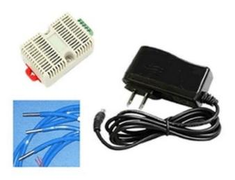
SM1210B-12 using the standard RS485 bus MODBUS-RTU protocol, easy access to PLC DCS and other instruments or systems for monitoring temperature, humidity@12 state quantities. The internal use of high-precision sensing core and related devices to ensure high reliability and excellent long-term stability, can be customized RS232, RS485, CAN, 4-20mA, DC0~5V\10V, ZIGBEE, Lora, WIFI, GPRS and other output methods.
