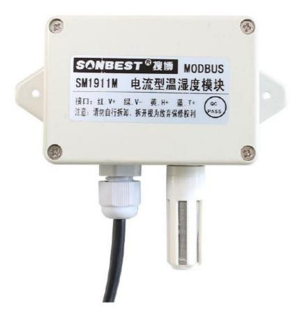
SM1911 using the standard ,easy access to PLC DCS and other instruments or systems for monitoring temperature, humidity state quantities. The internal use of high-precision sensing core and related devices to ensure high reliability and excellent long-term stability can be customized RS232, RS485, CAN,4-20mA, DC0~5V\10V, ZIGBEE, Lora, WIFI, GPRS and other output methods.
