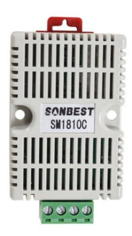
SM1810C using the standard CAN Bus, easy access to PLC DCS, and other instruments or systems for monitoring temperature, humidity state quantities. The internal use of high-precision sensing core and related devices to ensure high reliability and excellent long-term stability can be customized RS232, RS485, CAN,420mA, DC0~5V\10V, ZIGBEE, Lora, WIFI, GPRS, and other output methods.
