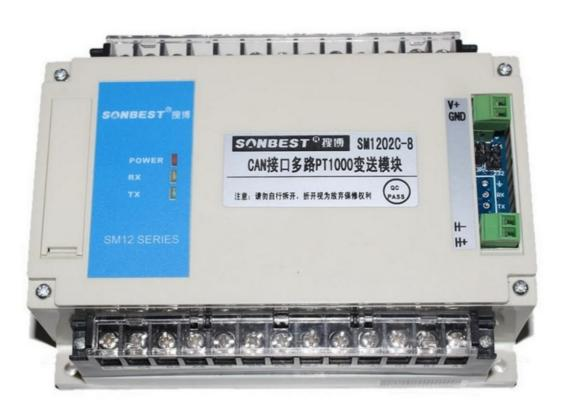
SM1202C using the standard CAN Bus, easy access to PLC DCS, and other instruments or systems for monitoring temperature@8 state quantities. The internal use of high-precision sensing core and related devices to ensure high reliability and excellent long-term stability can be customized RS232,RS485,CAN,4-20mA,DC0~5V\10V,ZIGBEE,Lora,WIFI,GPRS and other output methods.
