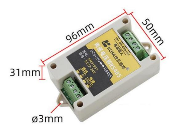
The distance between the two holes: is 86mm
