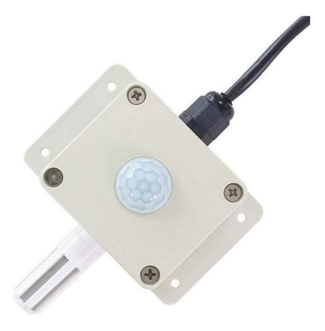
KM35B91 using the standard RS485 bus MODBUS-RTU protocol, easy access to PLC DCS, and other instruments or systems for monitoring Illuminance, temperature, and humidity state quantities. The internal use of high-precision sensing core and related devices to ensure high reliability and excellent long-term stability can be customized RS232, RS485, CAN,4-20mA, DC0~5V\10V, ZIGBEE, Lora, WIFI, GPRS and other output methods.
