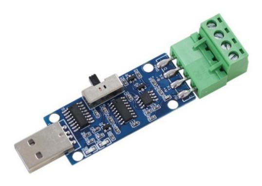
HD813 using the standard USB, easy access to PLC, DCS, and other instruments or systems for monitoring RS485, TTL state quantities. The internal use of high-precision sensing core and related devices to ensure high reliability and excellent long-term stability can be customized RS232, RS485, CAN,40mA, DC0~5V\10V, ZIGBEE,Lora, WIFI, GPRS, and other output methods.
