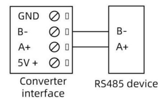
**Note:** When the power supply of the user equipment is DC5V, the converter can directly supply power to the user equipment, GND is the negative pole of the power supply, and 5V is the positive pole of the power supply. It can only supply power to devices with a power supply of 5V
