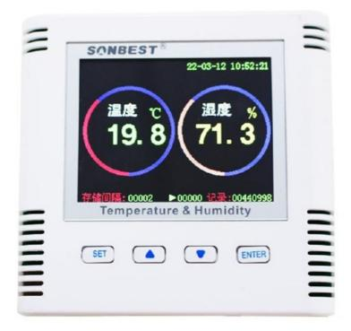
XR6813B using the standard RS485 bus MODBUS-RTU protocol, easy access to PLC DCS and other instruments or systems for monitoring temperature, humidity state quantities. The internal use of high-precision sensing core and related devices to ensure high reliability and excellent long-term stability, can be customized RS232, RS485, CAN, 4-20mA, DC0~5V\10V, ZIGBEE, Lora, WIFI, GPRS and other output methods.
