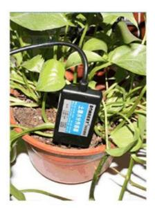
Choose a suitable measurement location, avoid rocks, cut the surface soil according to the depth required for measurement, maintain the original tightness of the underlying soil, hold the sensor vertically and insert it into the soil, do not shake left and right when inserting, to ensure close contact with the soil
