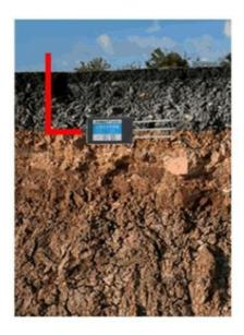
Dig a pit with a diameter of about 20cm vertically, insert the sensor needle into the pit horizontally according to the measurement needs, and fill the pit to ensure close contact with the soil. After the sensor is stable for a period of time, continuous long-term measurement and recording can be performed.
