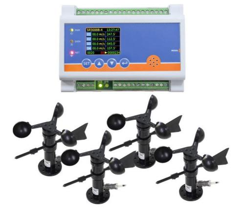
SR3688B using the standard RS485 bus MODBUS-RTU protocol, easy access to PLC DCS and other instruments or systems for monitoring wind speed, conductivity state quantities. The internal use of high-precision sensing core and related devices to ensure high reliability and excellent long-term stability, can be customized RS232,RS485,CAN,4-20mA,DC0~5V\10V,ZIGBEE,Lora,WIFI,GPRS and other output methods.
