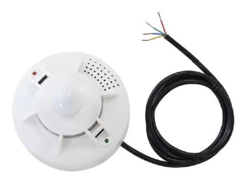
SM7590B uses the standard RS485 bus MODBUS-RTU protocol, easy access to PLC DCS, and other instruments or systems for monitoring carbon dioxide, temperature, humidity, illuminance, noise state quantities. The internal use of high-precision sensing core and related devices to ensure high reliability and excellent long-term stability can be customized RS232, RS485, CAN,4-20mA, DC0~5V\10V, ZIGBEE, Lora, WIFI, GPRS and other output methods.
