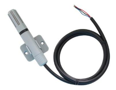
SM7320V using the standard DC0 ~ 5V voltage output signal, easy access to PLC DCS, and other instruments or systems for monitoring humidity state quantities. The internal use of high-precision sensing core and related devices to ensure high reliability and excellent long-term stability can be customized RS232, RS485, CAN,4-20mA, DC0~5V\10V, ZIGBEE, Lora, WIFI, GPRS, and other output methods.
