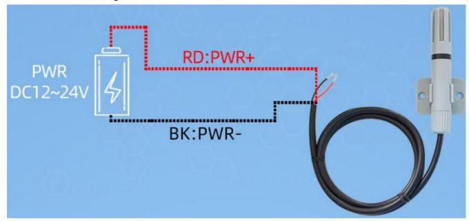
• Current three – wire wiring
