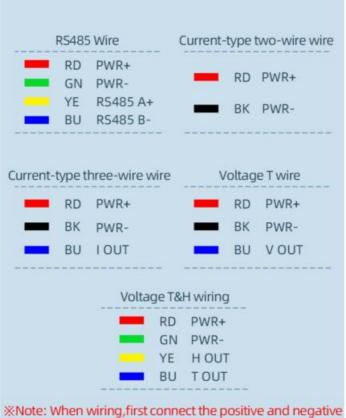
poles of the power supply, and then connect the signal line
