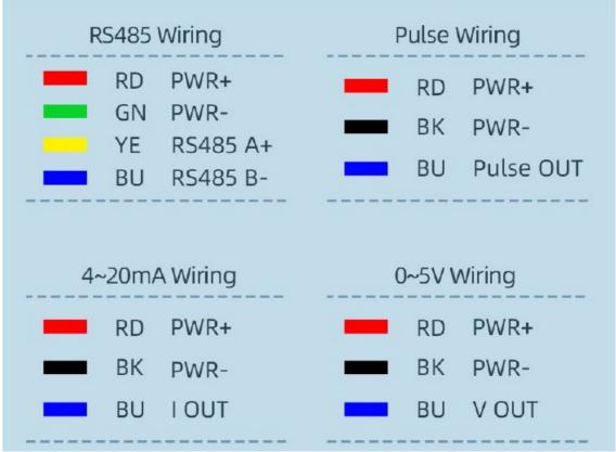
Note: Connect the positive and negative poles of the power supply first, then connect the signal line
