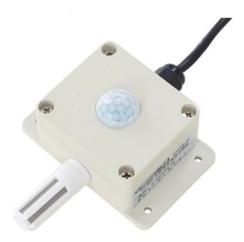
SM3590B using the standard RS485 bus MODBUS MODBUS-RTU protocol, easy access to PLC PLC DCS and other instruments or systems for monitoring illuminance, temperature, humidity state quantities. The internal use of high high-precision sensing core and related devices to ensure high reliability and excellent long long-term stability can be customized RS232, RS485, CAN, 4 4-20mA, DC0~5V 5V\10V, ZIGBEE, Lora, WIFI, GPRS and other output methods.
