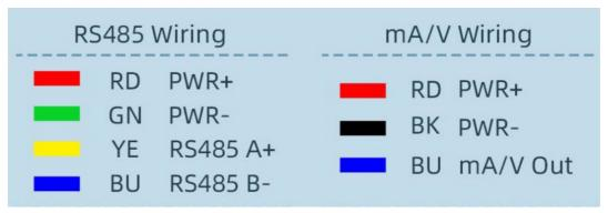
**NOTE**: When the wiring , the positive and negative poles of the power supply are connected first , and then the signal line.
