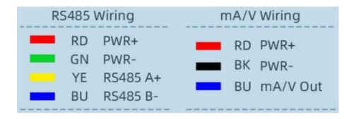
**Note:** When wiring, the positive and negative poles of the power supply are connected first, and then the signal line.
