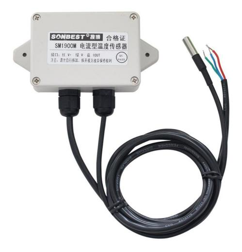
SM1900M using the standard DC4-20mA current output signal, easy access to PLC DCS, and other instruments or systems for monitoring temperature state quantities. The internal use of high -precision sensing core and related devices to ensure high reliability and excellent long-term stability, can be customized RS232, RS485, CAN,4-20mA, DC0~5V\10V, ZIGBEE, Lora, WIFI, GPRS and other output methods.
