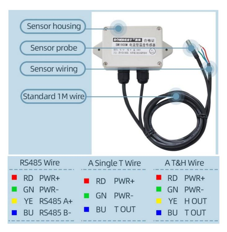
**Note:** When wiring, first connect the positive and negative poles of the power supply, and then connect the signal line.
