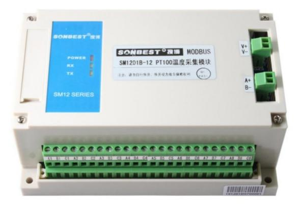
SM1201B-12 using the standard RS485 bus MODBUS-RTU protocol, easy access to PLC DCS, and other instruments or systems for monitoring temperature@12 state quantities. The internal use of high-precision sensing core and related devices to ensure high reliability and excellent long-term stability can be customized RS232, RS485, CAN,4-20mA, DC0~5V\10V, ZIGBEE, Lora, WIFI, GPRS and other output methods.
