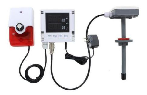
SD6788B uses the standard, easy access to PLC DCS, and other instruments or systems for monitoring wind speed, temperature, humidity, RS485 state quantities. The internal use of high-precision sensing core and related devices to ensure high reliability and excellent long-term stability can be customized RS232, RS485, CAN,4-20mA, DC0~5V\10V, ZIGBEE, Lora, WIFI, GPRS, and other output methods.
