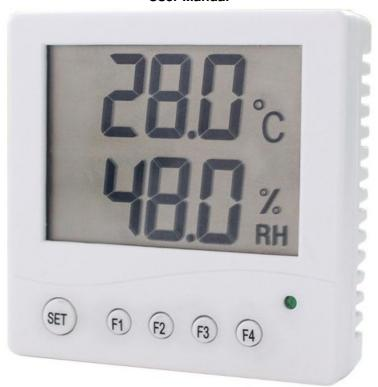
SD5110B uses the standard RS485 bus MODBUS-RTU protocol, easy access to PLC, DCS, and other instruments or systems for monitoring temperature, and humidity state quantities. The internal use of high-precision sensing core and related devices to ensure high reliability and excellent long-term stability can be customized RS232, RS485, CAN,4-20mA, DC0~5V\10V, ZIGBEE, Lora, WIFI, GPRS and other output methods.
