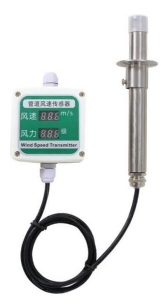
SD3789B using the standard RS485 bus MODBUS-RTU protocol, easy access to PLCDCS and other instruments or systems for monitoring wind speed state quantities. The internal use of high -precision sensing core and related devices to ensure high reliability and excellent long-term stability, can be customized RS232, RS485, CAN, 4-20mA, DC0~5V10V, ZIGBEE, Lora, WIFI, GPRS and other output methods.
