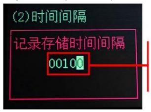
Press the second "SET" to enter the storage interva I setting The upper limit can be set to 100 seconds/time
