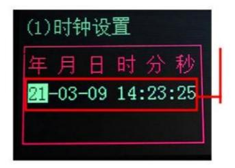
Press "SET" to enter the clock setting Use to shift, adjust the value up and down
