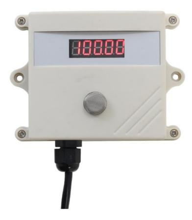
SD2130M-NH3 using the standard DC4-20mA current output signal, easy access to PLC DCS and other instruments or systems for monitoring ammonia state quantities. The internal use of high -precision sensing core and related devices to ensure high reliability and excellent long-term stability, can be customized RS232,RS485,CAN,4-20mA,DC0~5V\10V,ZIGBEE,Lora,WIFI,GPRS and other output methods.
