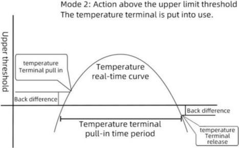
The temperature terminal pull-in action condition: measured value>upper limit threshold + return difference value
