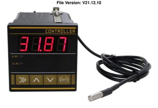
SC7200B using the standard RS485 bus MODBUS-RTU protocol, easy access to PLC, DCS, and other instruments or systems for monitoring temperature state quantities. The internal use of high-precision sensing core and related devices to ensure high reliability and excellent long-term stability can be customized RS232, RS485, CAN,4-20mA, DC0~5V\10V, ZIGBEE, Lora, WIFI, GPRS and other output methods.
