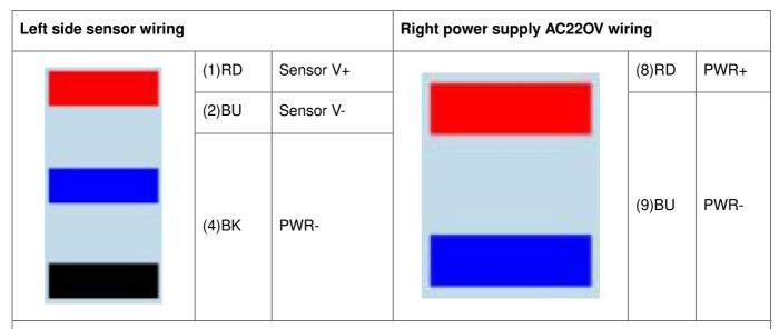
Note: When wiring, connect the positive and negative poles of the power supply first, and then connect the signal wire
