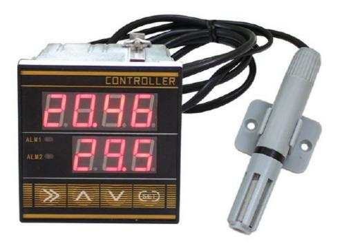
SC7210B u sing the standard RS485 bus MODBUS RTU protocol,easy access to PLC DCS and other instruments or systems for monitoring temperature, humidity state quantities. The internal use of high precision sensing core and related devices to ensure high r eliability and excellent long term stability, can be customized RS232,RS485,CAN,4 20mA,DC0~5V 10V,ZIGBEE,Lora,WIFI,GPRS and other output methods.
