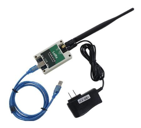
QU9192L using the standard USB,easy access to PLC DCS and other instruments or systems for monitoring LORA state quantities. The internal use of high-precision sensing core and related devices to ensure high reliability and excellent long-term stability, can be customized
