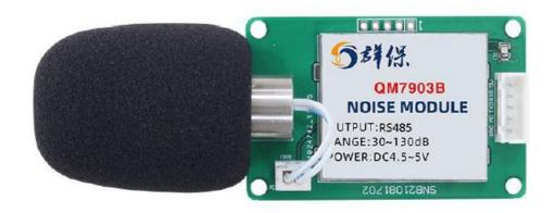
QM7903B using the standard ,easy access to PLC DCS and other instruments or systems for monitoring noise state quantities. The internal use of high-precision sensing core and related devices to ensure high reliability and excellent long-term stability, can be customized RS232,RS485,CAN,4-20mA,DC0~5V\10V,ZIGBEE,Lora,WIFI,GPRS and other output methods.
