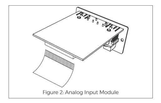
• Carefully insert the Analog Input Module into the amplifier being certain not to dislodge any components as you insert the module. Install the two screws that secure the module to the chassis.
