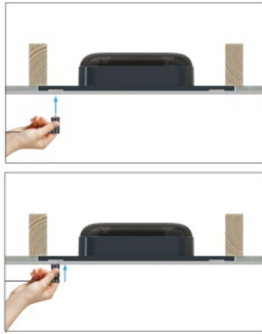
Figure 4: Placing the measurement probe
