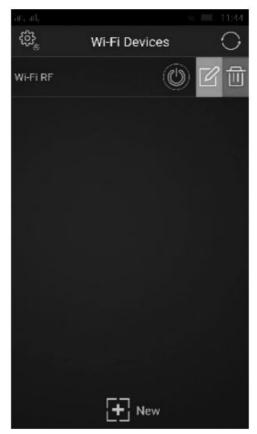
7. Once the connection has been made, the WiFi socket will be visible in the application. You can switch it ON / OFF or by sliding left you can edit, delete the device with the appearing icons.
