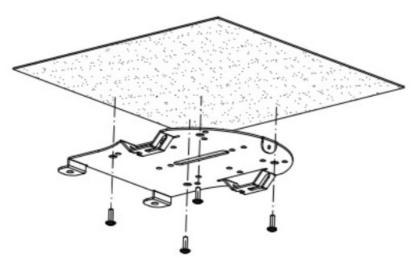
**Step 3.**Secure bottom component of mount to the bottom of the camera, using included M3\*6 screws.
