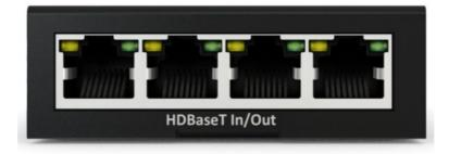
• HDBaseT input / output ports (x 4) – connect to Cat cable to transmitter/s or receiver/s
