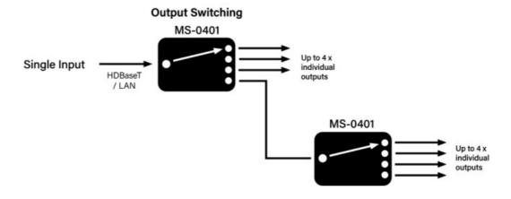
Networks and HDBaseT connectivity can be expanded using multiple MS-0401 units inline between point of transmission to receive. Adding in a subsequent MS-0401 unit will provide connectivity to up to 7 x displays from a single source. Cascading can also work for extra inputs.
