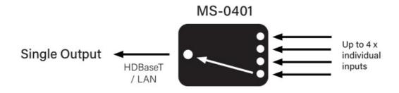
The MS-0401 can also be used to route any of up to 4 x input signals to the output.
