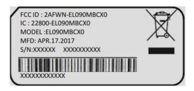
Product information is indicated in a printed sticker label. The information consists of Model (model name), MFD(manufacturing date), S/N(serial number)
