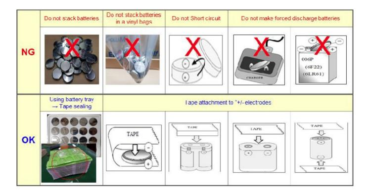
Proper use of battery tray is outlined below. With batteries properly placed into each tray slot stack the trays in the same orientation use an empty tray on the top stack tape the stack together to avoid falling apart.
